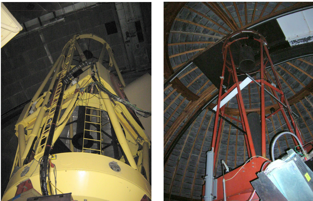
Figure 2. The 3-m Shane reflector and the 1-m Nickel reflector have human operators who compensate for pointing problems.
